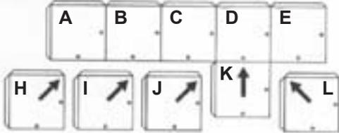
3. In the same way, install the remaining panels in the first row. Keep all panels carefully aligned and tight together.
